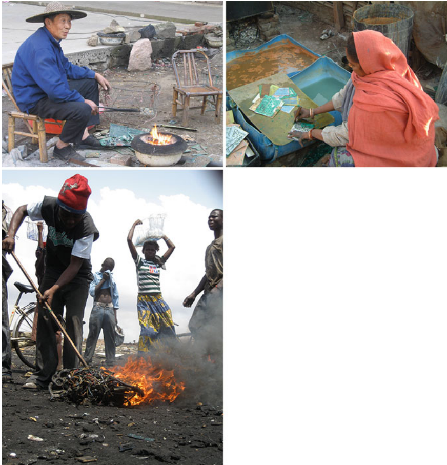
Fig. 2 Typical recycling processes applied in the informal sector of developing countries (left to right: de-soldering of printed wiring boards, leaching of copper from printed wiring boards, open burning of cables) (Pictures: Empa)
